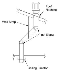
Figure 31 - Offset with Wall Strap and 45° Elbows
